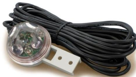
The advanced optical sensor uses infrared light to detect water hitting its surface. This method of detection is more sensitive and reliable than other methods, is nearly immune to false detection, and is not affected by movement and most environmental conditions.
